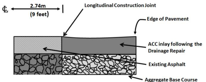
(Fig. 1) Outer Edge of pavement following the drainage repair and prior to final repair showing the construction joint and settlement.
