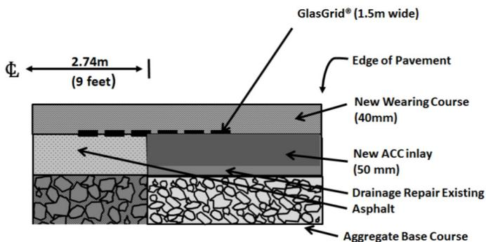
(Fig. 2) Outer Edge of pavement following final repair using GlasGrid® 8502
