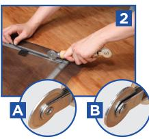
2. A: For aluminum screen, use the convex end of screen tool to gently roll screen into the frame groove to crease the screen.
